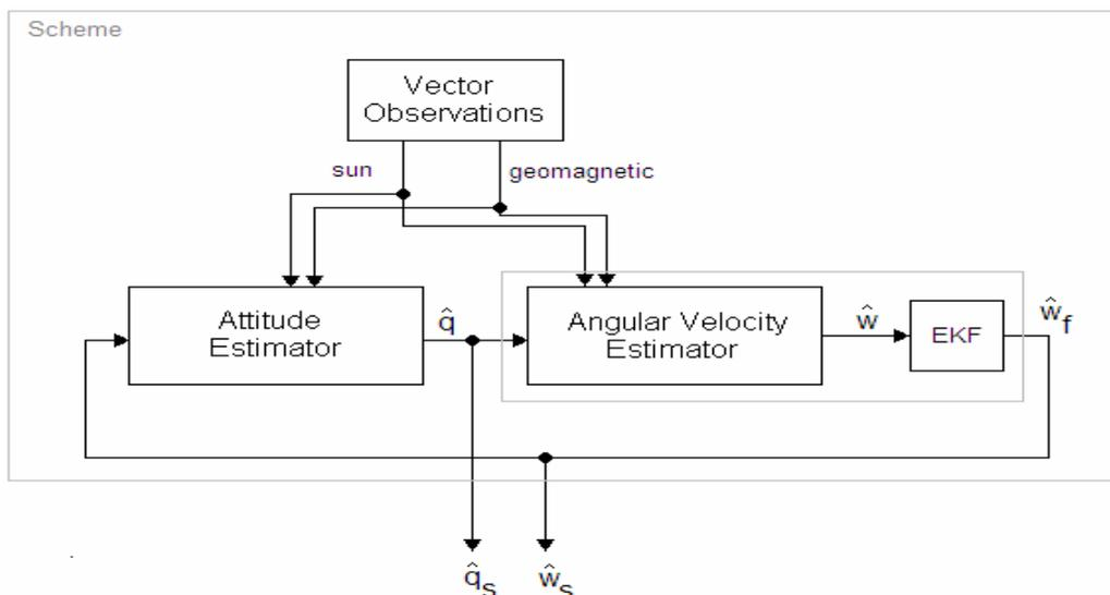
Figure 1 – Intertwined scheme for attitude/rate estimation.
