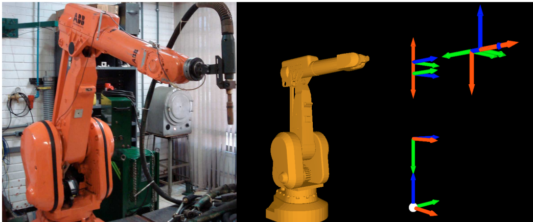
Figure 7. IRB2000 and its 3D representation
