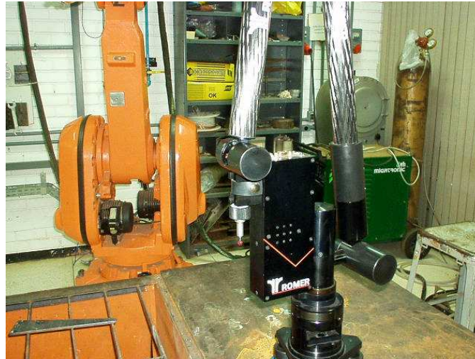
Figure 2. ITG ROMER measurement arm
