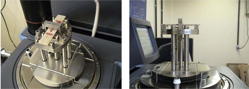
Figure 4. DMA 3-Point Bending Test
