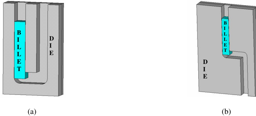
Figure 4. Three dimensional FEM model employed in the ECAP simulation corresponding to: (a) route A; (b) route C.
