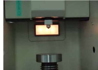
At left the Hardness Calibration Machine SHT-31. At right and upper picture the SHT-31 operation panel, and At right and lower picture details of Indenter and measurement anvil.
