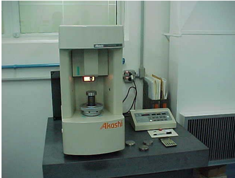
At left the Hardness Calibration Machine SHT-31. At right and upper picture the SHT-31 operation panel, and At right and lower picture details of Indenter and measurement anvil.
