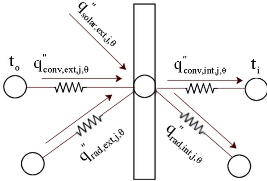
Figure 2. Schematics of heat balance processes in a single pane window
