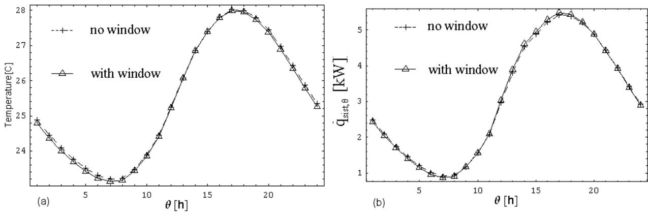
Figure 6. Effect of accounting the window balance equation: (a) temperature distribution; (b) equipment cooling load
