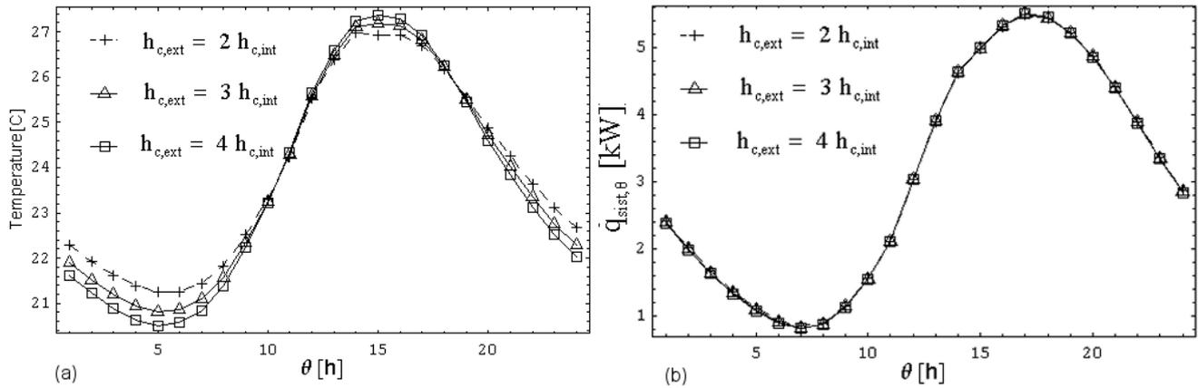
Figure 8. Effect of the relation between convective coefficients: (a) window temperature, (b) equipment cooling load
