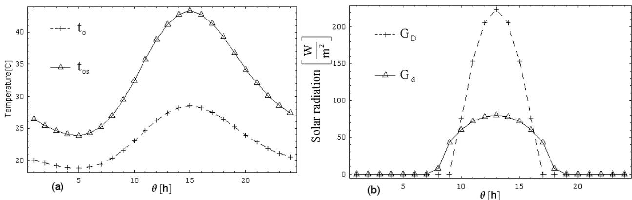
Figure 4. Temperature and radiation distributions: (a) outside surface and outdoor temperature, (b) direct and diffuse solar radiation
