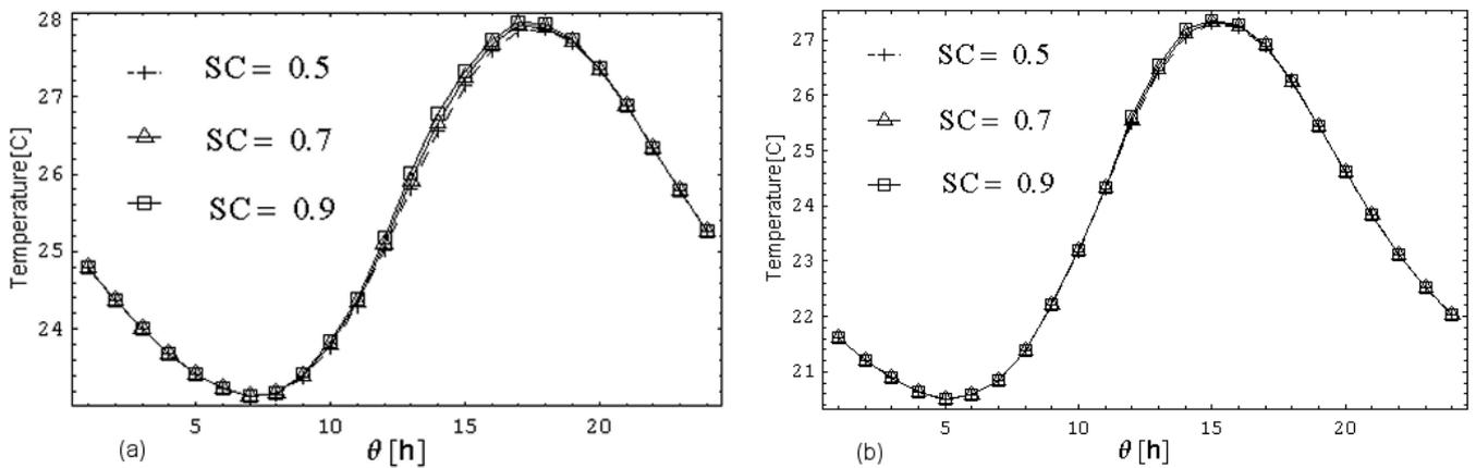
Figure 7. Effect of the shadow coefficient on temperature distribution: (a) wall, (b) window
