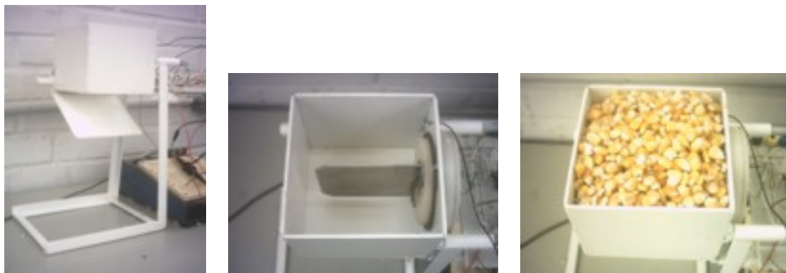
Figure 1. Moisture Sensor final mechanical conception(Lagares and Sousa, 2006)
