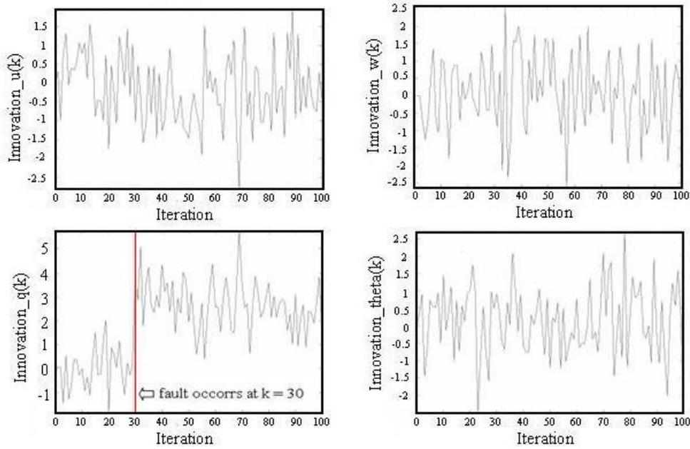
Figure 5. Kalman Filter innovation process in the case pitch rate gyro fault.
