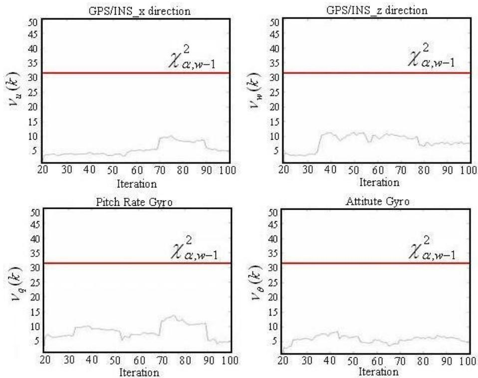
Figure 4. Fault Diagnosis: behaviour of  $v_i(k)$  when there is no sensor fault in the system.
