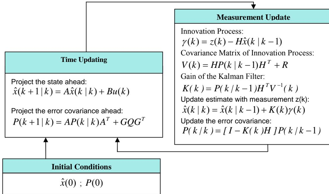
Figure 1. Kalman Filter Algorithm
