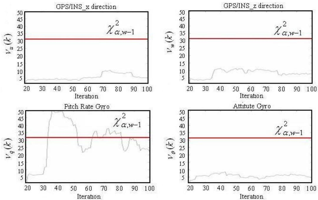
Figure 7. Behaviour of  $v_i(k)$  in the case pitch rate gyro fault.
