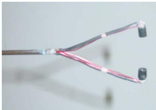
Figure 2 – Probe containing the pair of emitter-detector optic devices, corresponding to a light emitting diode (LEDs) and a photo-transistor as the sensors.
