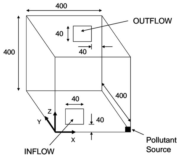
Figure 1 – Schematic diagram of the experimental cubic chamber (dimensions are in millimeters)
