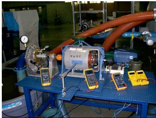
Figure 6. Experimental setup employed to determine the turbine performance characteristics.
