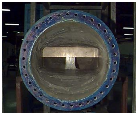
Figure 9. Picture of the mechanical gate offering 43.75 % of restriction for the water flowing out from the tailrace pipe.
