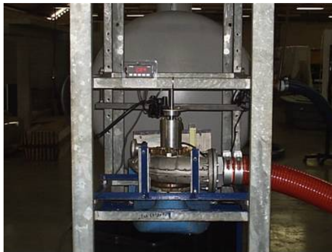
Figure 1. Frontal picture of the vertical Francis turbine installed at its test bench.
