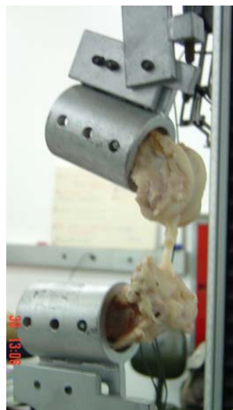
(b) ACL deformation during the tensile tests.
