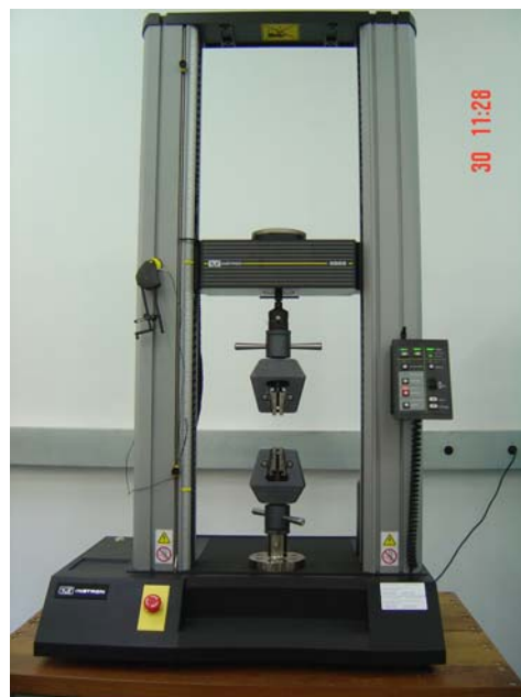
Figure 1. Universal materials testing Instron machine, model 5869, from the physical tests laboratory at CETEC-MG.
