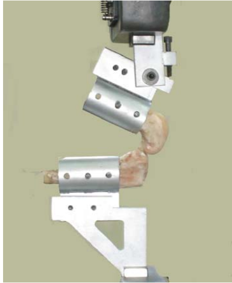
Figure 2. Picture of the gripping system specially devised to test ACL specimens with bone ends.
