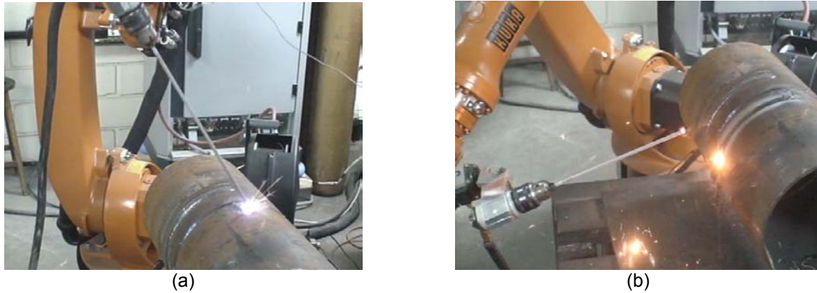
Figure 13. Robot positioning at initial (a) and end points (b) for an orbital welding.
