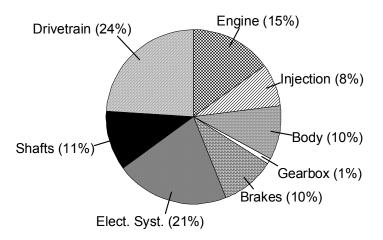
Figure 3. Distribution of component failures - Argentina
