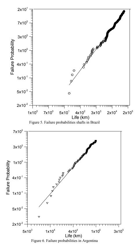
The values of the Weibull shaper parameters of all mechanical components are summarized in Table 1. Shaper parameter smaller than unity ( $\beta < 1$ ) means that after an initial large value, the failure rate decreases with
