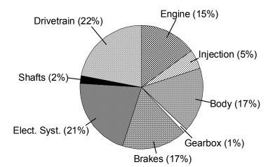
Figure 2. Distribution of component failures - Brazil
