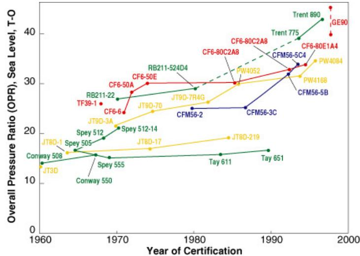
**Figure 4** Pressure ratio trends for commercial transport engines (Jane's, 2001).
