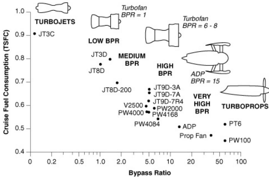
**Figure 5:** Trends in engine bypass ratio (Jane's, 2001)
