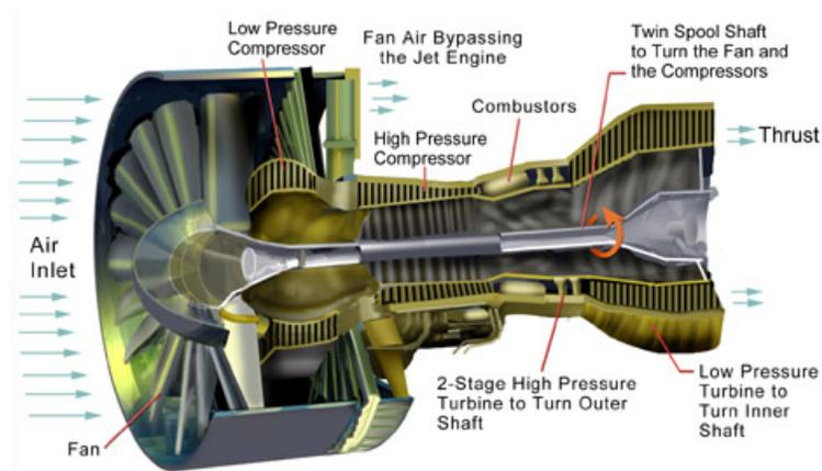
**Figure 2:** A typical high bypass-ratio turbofan (Adapted from Pratt & Whitney, MIT Notes Lectures (2005)).
