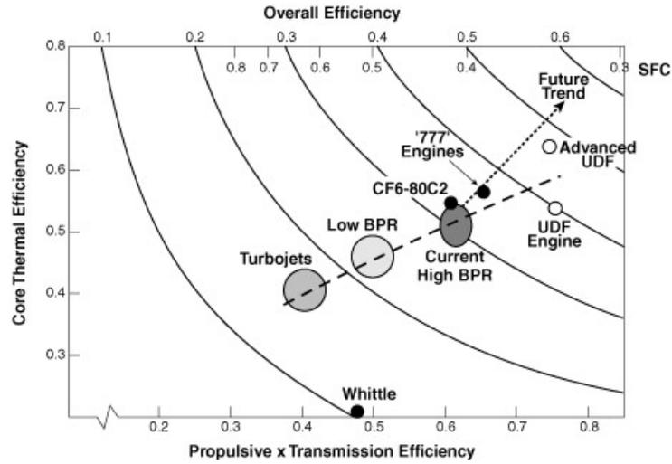
**Figure 3:** Trends in aircraft engine efficiency (after Pratt & Whitney).
