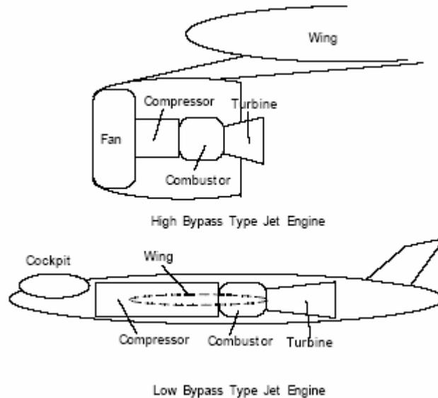
**Figure 1:** Schematic Comparison of Architectures of Two Types of Jet Engines (Crawley et al, 2004)
