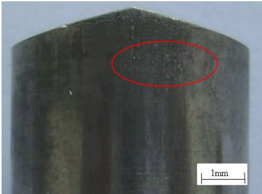
Figure 12 – Lateral Wear of the Punch Tool P4 .
