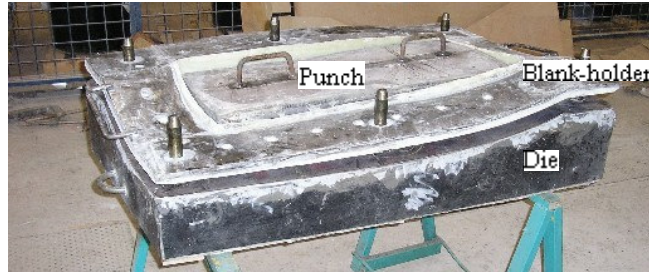
Figure 1: Base, punch and blank-holder. Foroni (2005).
