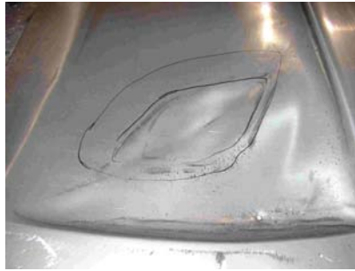
Figure 4. Sheet 3 after conformation. Feroni (2005).
