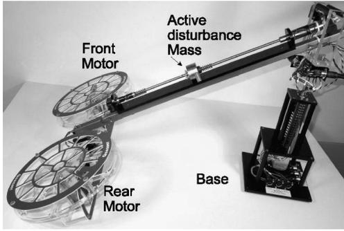
Figure 1. Helicopter with Active Disturbance Mass.
