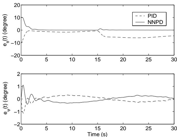
Figure 6. Tracking error of the pitch and yaw angles.
