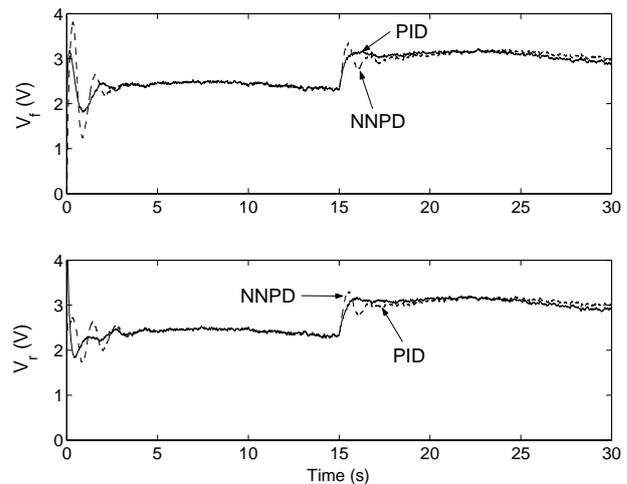
Figure 7. Control input signals of the helicopter.
