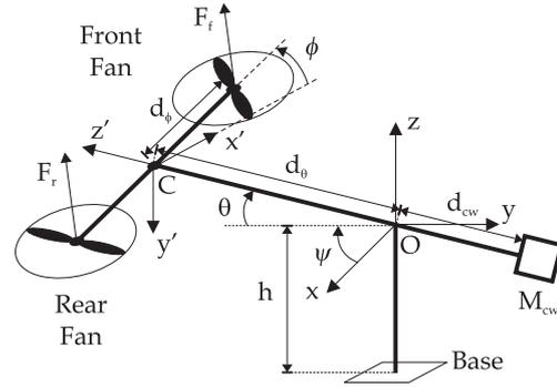
Figure 2. Tandem Fan in a 3 DOF Platform.
