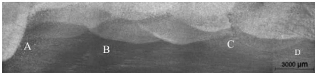
Figure 10. CGHAZ extension with energy ratio 5/5 kJ/cm with PWHT.
