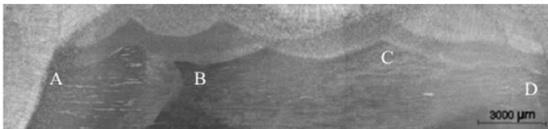
Figure 8. CGHAZ extension with the energy ratio 5/5 kJ/cm without PWHT.
