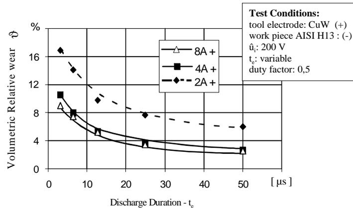
Figure 5. Volumetric relative wear  $\vartheta$  with the variation of discharge current  $i_e$  and discharge duration  $t_e$  for EDM with positive Copper-Tungsten electrodes.
