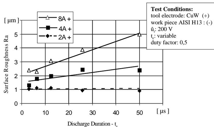
Figure 6. Results of surface roughness  $R_a$  when EDM using Copper-Tungsten electrodes at positive polarity.
