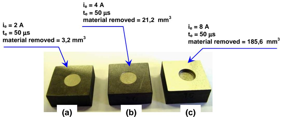
Figure 4. AISI H13 samples after EDM with positively charged CuW tool electrodes under  $\hat{i}_e =$  (a) 2 A (b) 4 A and (c) 8 A at optimum  $t_e = 50$  applying isoenergetic generator mode.
