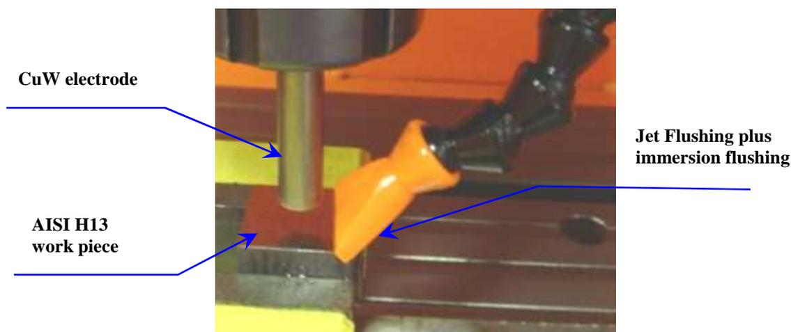
Figure 1. The picture depicts the assembly of electrode, work piece and the flushing method.
