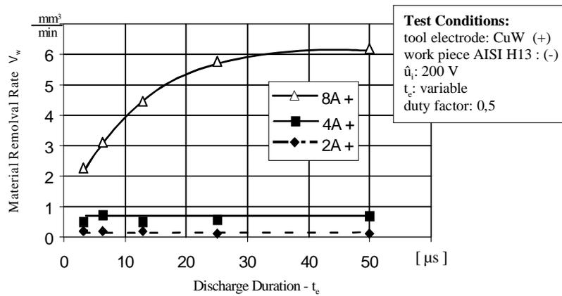
Figure 3 . Material removal rate  $V_w$  with variation of discharge current  $\hat{i}_e$  and discharge duration  $t_e$  for EDM with positive Copper-Tungsten electrodes.
