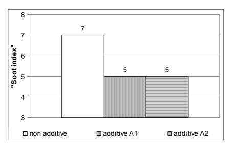
Figure 10. Effect of additives on "soot index" of flue gases (furnace test)
