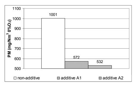
Figure 9. Effect of additives on PM emissions (furnace test)
