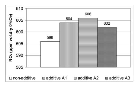
Figure 4. Effect of additives on NO<sub>x</sub> emissions (test boiler)
