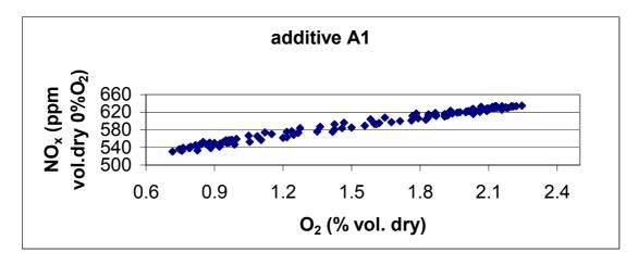
Figure 3. Effect of air excess on CO and NO<sub>x</sub> emissions (boiler test)
