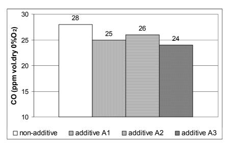
Figure 5. Effect of additives on CO emissions (test boiler)
