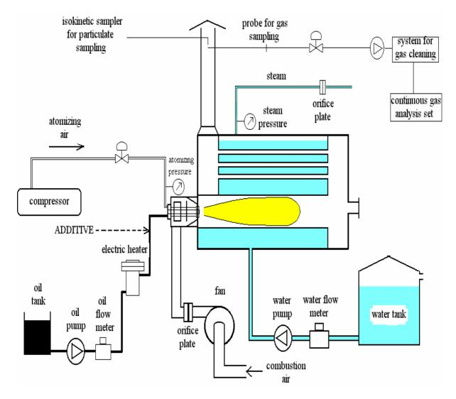
Figure 2. Test boiler schematic drawing (basic flowsheet of the test furnace is similar)
