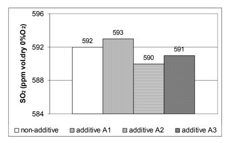
Figure 6. Effect of additives on SO<sub>2</sub> emissions (boiler test)
