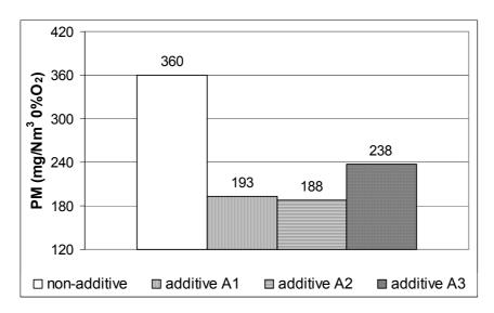
Figure 7. Effect of additives on PM emissions (boiler test)
