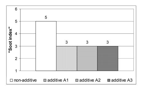
Figure 8. Effect of additives on "soot index" of flue gases (boiler test)
