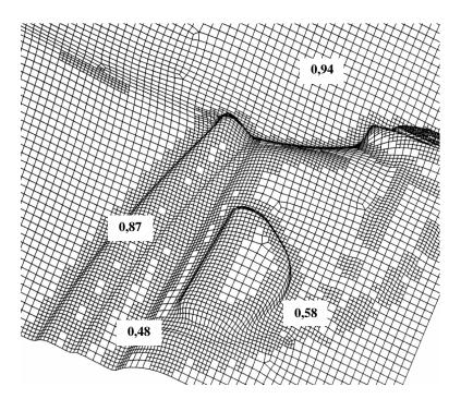
Figure 6. Thickness distribution after deformation in the step 2
