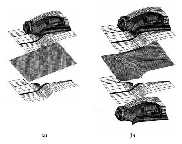
Figure 3. Forming stages 1 and 2 discretization models.
