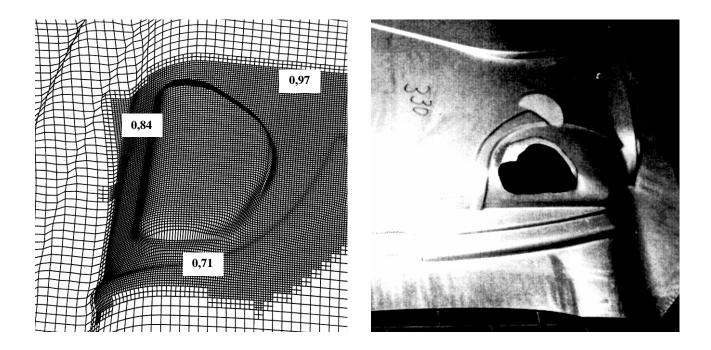
Figure 7 - (a) Thickness distribution after deformation in the step3 (tool radius optimization) and (b) prototype pressed body-in-white part.
