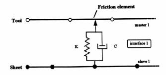
Figure 1. Mechanical equivalent contact force algorithm
