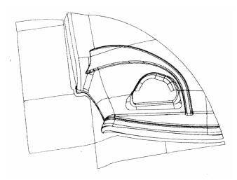
Figure 2. Critical area of a body-in-white side panel outer
