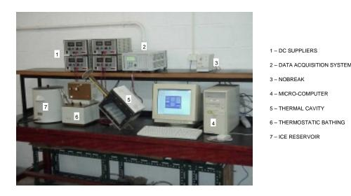
Figure 5. Photo of the experimental assembly for temperature measurements in the thermal cavity.
