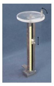
Figure 4. Thermocouple probes and positioning system for temperature measurements inside the cavities.
