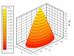
Figure 6 - Velocity profile for flow of dilatant fluid with behavior index, n = 5, inside a duct with aspect ratio,  $\rho_{asp} = 0.5$ .
