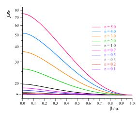
Figure 3 – Fanning friction factor *fRe* as function of the aspect ratio,  $\rho_{asp}$ , and behavior index, n.
