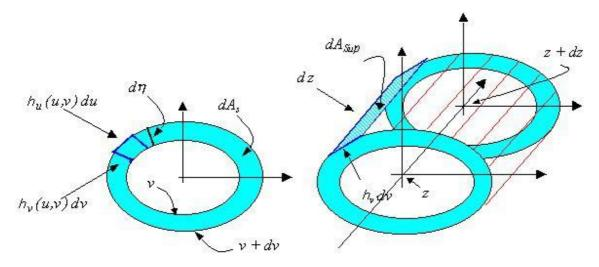
Figure 2. – Visualization of elliptical and axial differential elements having areas  $dA_s$  and  $dA_{Sup}$  in order to determine pressure and shear stress forces.
