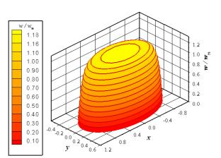
Figure 4 – Velocity profile for flow of pseudoplastic fluid with behavior index, n = 0.1, inside a duct with aspect ratio,  $\rho_{asp} = 0.5$ .
