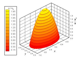
Figure 5 - Velocity profile for flow of Newtonian fluid with behavior index, n = 1, inside a duct with aspect ratio,  $\rho_{asp} = 0.5$ .
