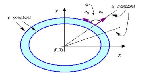
Figure 1. Non-orthogonal coordinate system (u, v).
