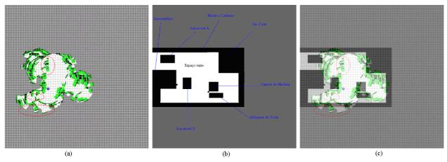
Figure 5 – (a)Graco's map obtained through the developed system, (b)Graco's manual map and (c)Maps superimposed.
