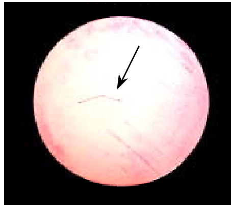
Figure 9. Crack detected by liquid penetrant testing.
