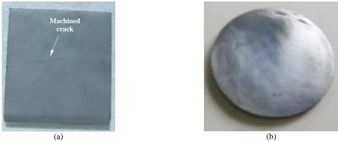
Figure 1. Test samples of ASTM A 36 steel plate (a) and AISI 1045 steel round bar (b).
