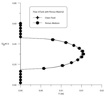
Figure 4 - Velocity profiles at the exit of a tank for porous medium with cF = 0.0, = 0.998 and  $K = 1 \times 10^{10} m^2$
