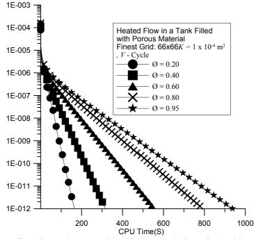
Figure 8 – Effect of Porosity  $\phi$  on residue history of velocity U for 4-grids, Re<sub>in</sub> = 300.
