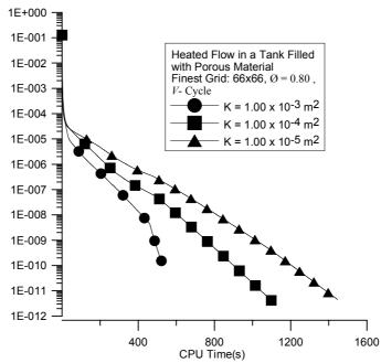
Figure 7 - Effect of Permeability K on residue history of Temperature T for 4-grids,  $Re_{in} = 300$ .
