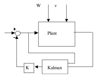
Figure 3. LQR Control Scheme with optimum state observer
