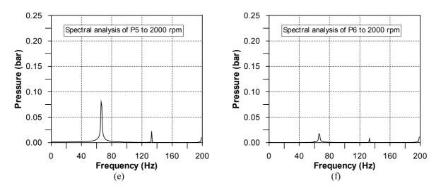
Figure 8- Pressure from transducers P1 (a), P2 (b), P3 (c), P4 (d), P5 (e) and P6 (f) versus frequency for configuration H at 2000 rpm.
