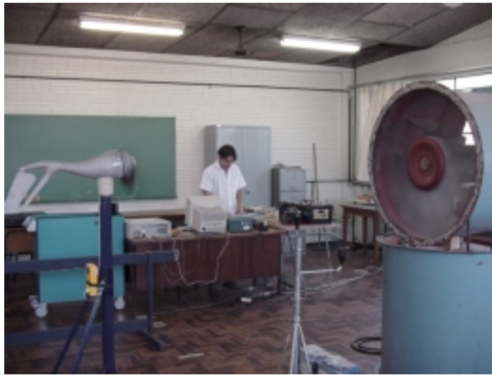
Figure 10: Test in laboratory of a 400W SWTG.
