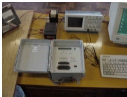
Figure 9: Detail of bench test showing data logger and power transducer.
