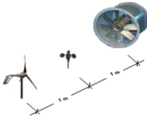
Figure 5: Scheme of separation between turbine, anemometer e axial fan.
