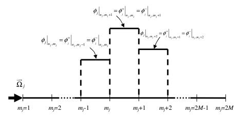
Figure 1- Representation of the radiation intensities for the discontinuous finite element formulation.
