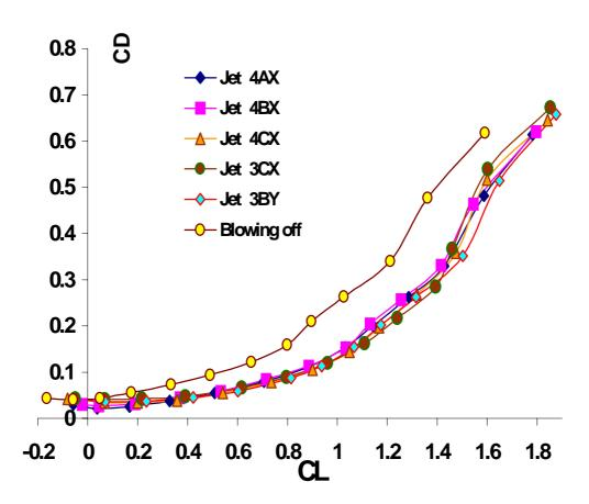
Figure 13 Drag polar for Triple Jets.
