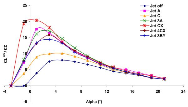
Figure 14 maximum range factor results of the best configurations.
