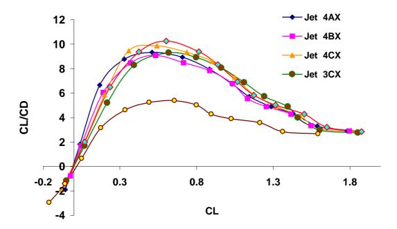
Figure 12 Wing efficiency with Triple Jets.
