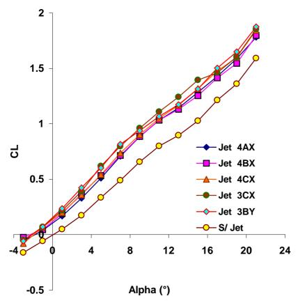
Figure 11 Lift curves for Triple Jets.
