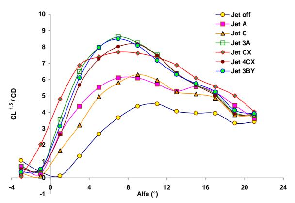
Figure 15 Climb rate factor results of the best configurations.
