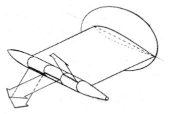
Figure 1 Three Wing Tip "Coanda" jets.
