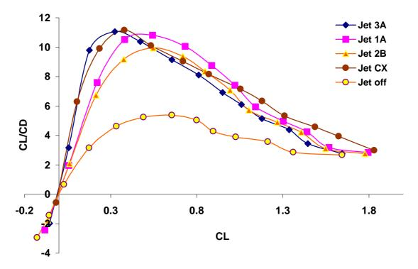
Figure 10 Wing efficiency with Double jets.
