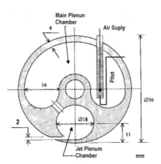
Figure 3 Jet module geometry and dimensions.
