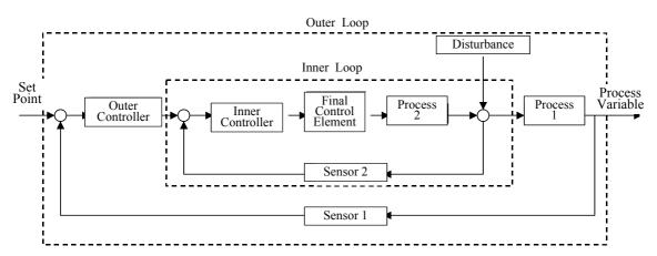
Figure 1. Cascade control architecture scheme.
