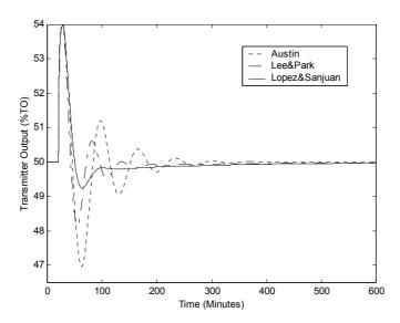
Figure 6. Process response for example 2, measured in transmitter output for a disturbance step change using a PI-PI cascade control architecture.
