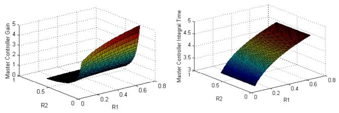
Figure 2. Response surfaces for master controller proportional gain and master controller integral time based on the tuning equations set found to PI-P cascade architecture.
