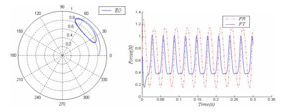
Figure 5. Case III:  $\varepsilon = 0.8$ , W = 33.6 kg, c = 2.54e-4 m,  $r_b = 2.54e-2$  m, L = 5.08e-2 m,  $F_u = 100$  N,  $V_b = 2000$  rpm,  $\eta = 8.276e-3$  Ns/m<sup>2</sup>.
