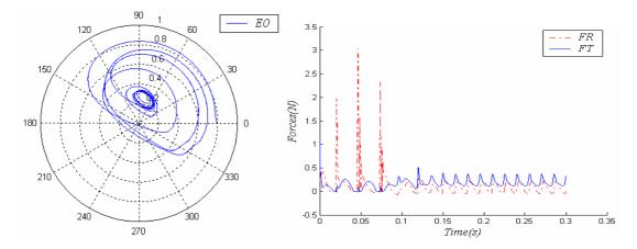
Figure 9. Case VII:  $\varepsilon = 0.8$ , W = 33.6 kg, c = 2.54e-4 m,  $r_b = 2.54e-2$  m, L = 5.08e-2 m,  $F_u = 100$  N,  $V_b = 4000$  rpm,  $\eta = 2.53e-2$  Ns/m<sup>2</sup>.
