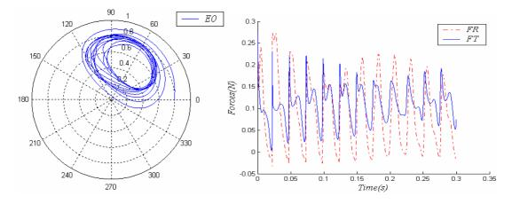
Figure 6. Case IV:  $\varepsilon = 0.8$ , W = 33.6 kg, c = 2.54e-4 m,  $r_b = 2.54e-2$  m, L = 5.08e-2 m,  $F_u = 100$  N,  $V_b = 5000$  rpm,  $\eta = 8.276e-3$  Ns/m<sup>2</sup>.
