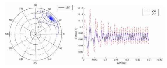
Figure 4. Case II:  $\varepsilon = 0.8$ , W = 33.6 kg, c = 2.54e-4 m,  $r_b = 2.54e-2$  m, L = 5.08e-2 m,  $F_u = 100$  N,  $V_b = 6000$  rpm,  $\eta = 2.622e-3$  Ns/m<sup>2</sup>.
