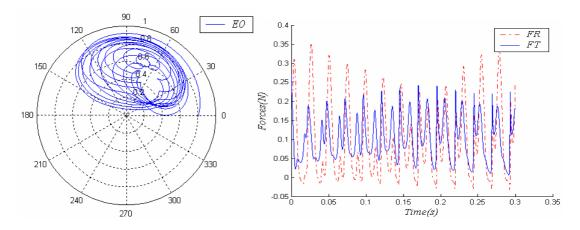
Figure 7. Case V:  $\varepsilon = 0.8$ , W = 33.6 kg, c = 2.54e-4 m,  $r_b = 2.54e-2$  m, L = 5.08e-2 m,  $F_u = 300$  N,  $V_b = 5000$  rpm,  $\eta = 8.276e-3$  Ns/m<sup>2</sup>.
