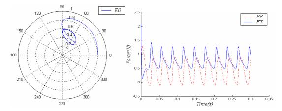
Figure 8. Case VI:  $\varepsilon = 0.8$ , W = 33.6 kg, c = 2.54e-4 m,  $r_b = 2.54e-2$  m, L = 5.08e-2 m,  $F_u = 100$  N,  $V_b = 2000$  rpm,  $\eta = 2.53e-2$  Ns/m<sup>2</sup>.
