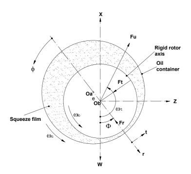
Figure 1. Squeeze film damper with dynamic forces and coordinates defined.
