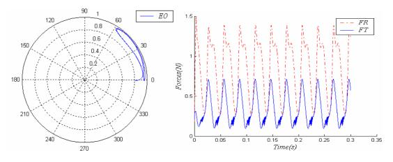
Figure 3. Case I:  $\varepsilon = 0.8$ , W = 33.6 kg, c = 2.54e-4 m,  $r_b = 2.54e-2$  m, L = 5.08e-2 m,  $F_u = 100$  N,  $V_b = 2000$  rpm,  $\eta = 2.622e-3$  Ns/m<sup>2</sup>.
