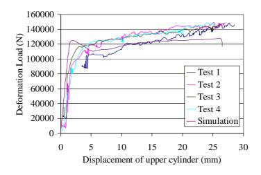
Figure 14. Deformation load tests and simulation.
