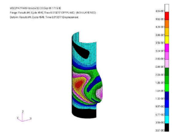
Figure 11. Effective strain distribution
