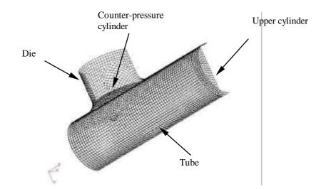
Figure 9. Finite element model.
