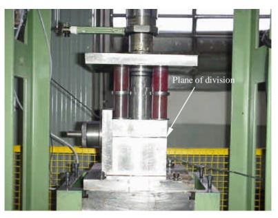
Figure 4. Hydroforming tools in the hydraulic press.
