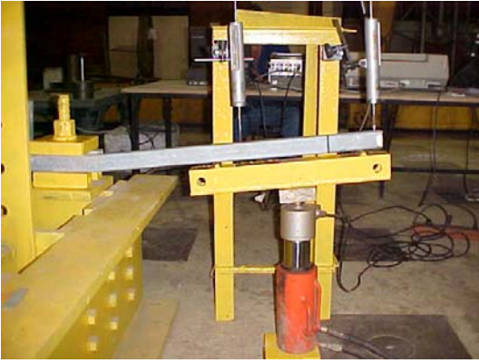
Figure 4. Track support test facility.
