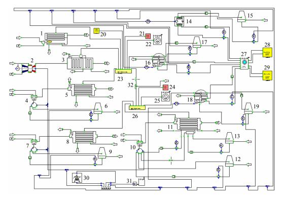
Figure 2. Configuration of the superstructure used in the structural and parametric optimization of a cogeneration system.
