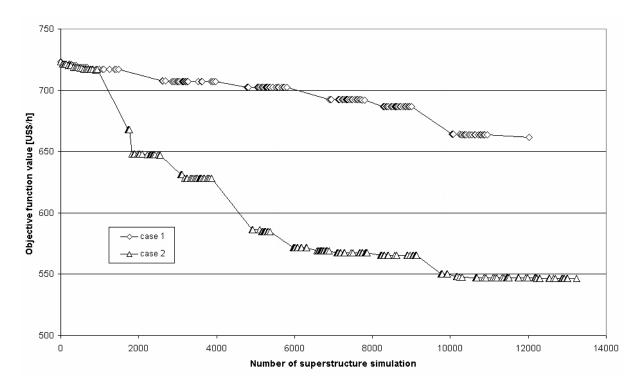
Figure 5. Objective function variation for Cases 1 and 2 throughout the optimization process of the superstructure shown in Fig. (2).
