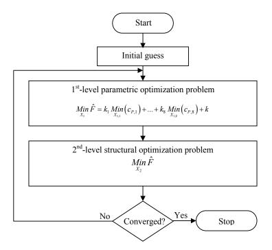
Figure 3. Iterative process for the multilevel optimization problem.
