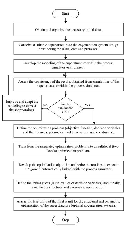
Figure 1. Basic stages of the optimization procedure.
