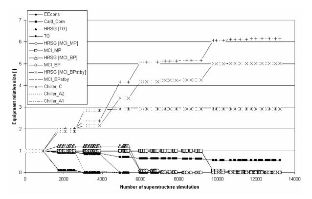
Figure 6. Evolution of the configuration of the cogeneration system for Case 2 throughout the optimization process of the superstructure shown in Fig. (2).
