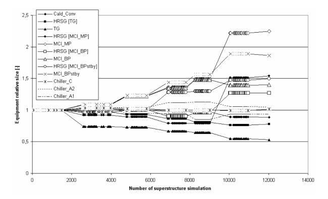
Figure 6. Evolution of the configuration of the cogeneration system for Case 1 throughout the optimization process of the superstructure shown in Fig. (2).
