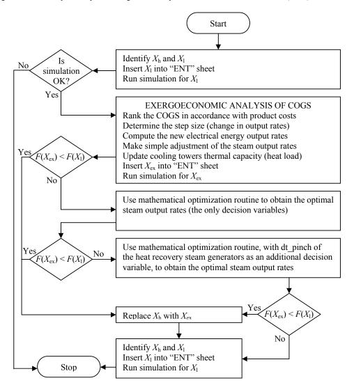
Figure 4. Logic based on an exergoeconomic analysis to assess the cogenerator subsystems (COGS).
