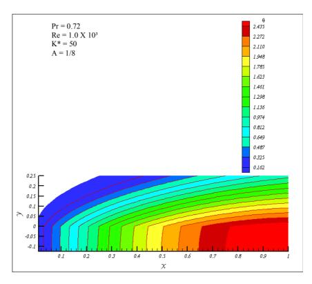
Figure 2 – Block and fluid temperature contours for a fourth-degree polynomial temperature and velocity approximations. Insulated surface condition at x = 1,  $k^* = 50$ , A = 1/8,  $Re = 1.0 \times 10^3$ .
