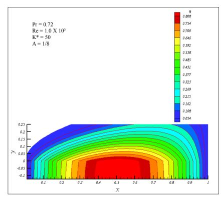
Figure 1 – Block and fluid temperature contours for a fourth-degree polynomial temperature and velocity approximations. Isothermal surface condition at x = 1,  $k^* = 50$ , A = 1/8,  $Re = 1.0 \times 10^3$ .
