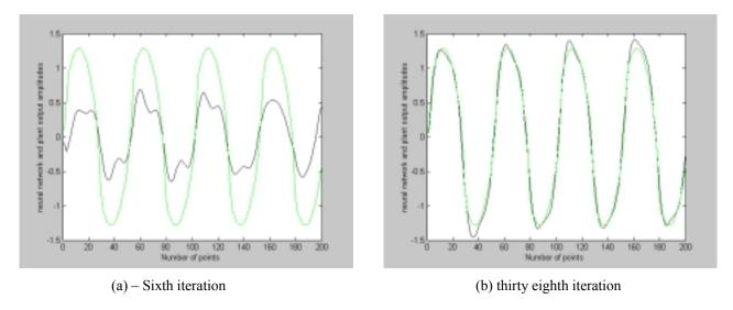
Figure 4. Output of the neural network (black) output of the plant (green)
