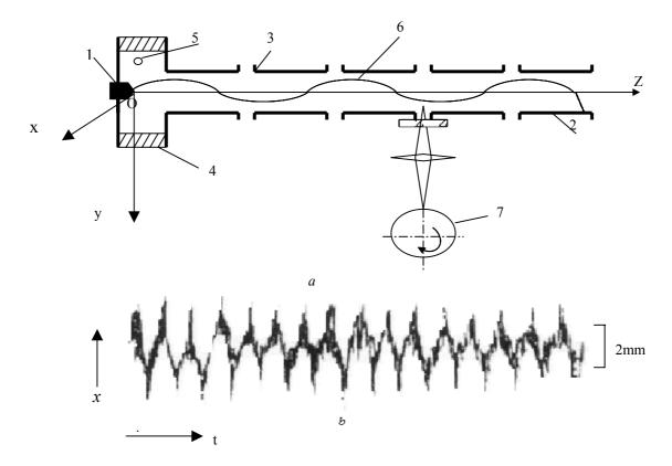
**Figure 1.** The experimental outline of the plasma generator (a) and a typical behavior of the electric arc oscillations for z = 8.5 cm, I = 200 A and G = 6 g/s (b).
