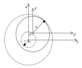
**Figure 3**. Scheme of the oscillations of the plasma arc; xOy is the laboratory system and x'O'y' is the arc coordinate system.
