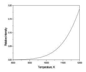
Figure 8. Relative intensity of the line Ar I 415.8 nm in function of the temperature
