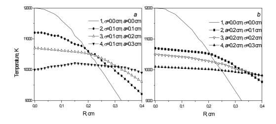
**Figure 9.** (9a) Radial distribution temperature for constant  $\sigma = 0.1$  cm and different values of a; (9b) Radial distribution temperature for constant a = 0.2 cm and different values of  $\sigma$ . The curve 1 corresponds the true radial temperature ( $\alpha = 0$ ,  $\sigma = 0$ ).
