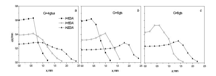
Figure 2. The experimental functions  $\varphi$  (x) for G = 4 g/s (a), 6 g/s(b) and 8 g/s (c), I = 100 A ( $\blacksquare$ ), I =150 A (O) and I =200 A ( $\triangle$ ).
