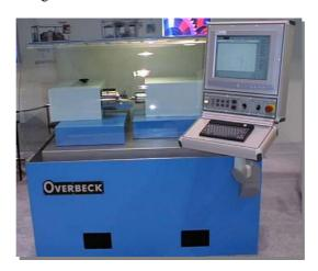
Figure 1 Overbeck® ID/OD grinding machine with PC-Based control..
