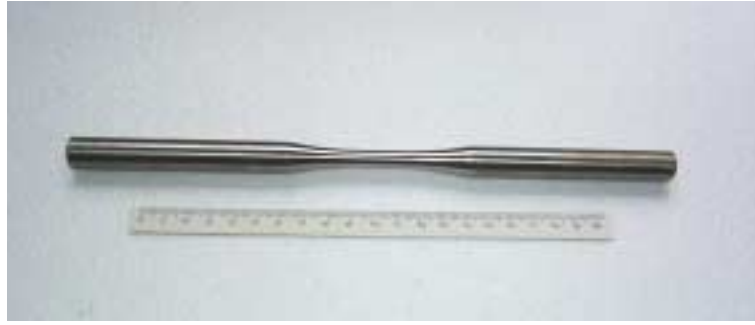
Figure 1. Test specimen of SAE 8620 steel used for damage studies.
