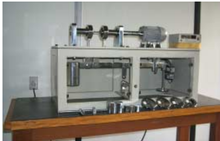
Figure 2. Rotating-bending fatigue testing machine used for damage studies.
