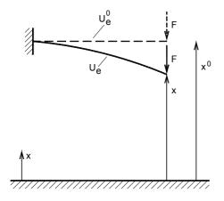
Figure 1 – Total Potential Energy written for a body in two different positions.
