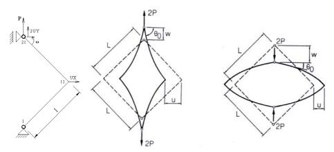
Figure 19 – Diamond frame, boundary conditons for tension and compression situations.
