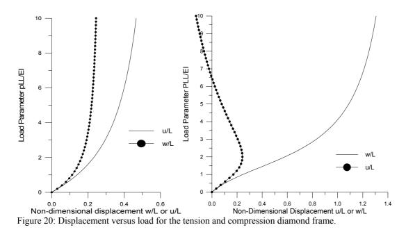
It has been used 20 finite elements to run the problem. In figures 20 and 21 the measured variables are numerically depicted, the reference value is not plotted because the maximum obtained error (in the last step for both tension and compression cases) are  $\varepsilon_{tension} = 1\%$  and  $\varepsilon_{compression} = 0.3\%$  when compared with the analytical solution
