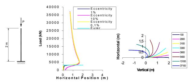
Figure - 9: Analyzed Column, lateral displacement and deformed shapes
