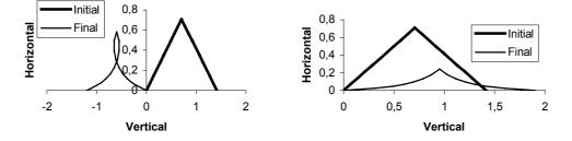
Figure 22 - Initial and final shapes for traction and compressed diamond frame
