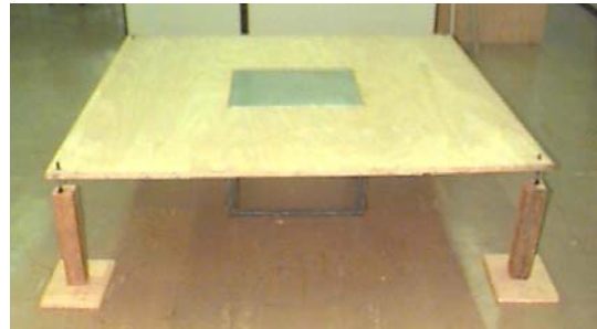
Figure 8. The plate mounted on a finite baffle.
