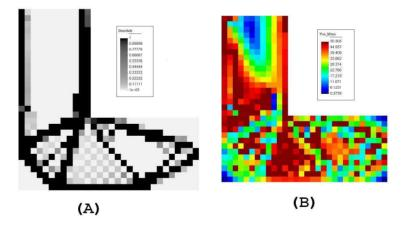
Figure 8. (A) Final topology. (B) Stress field ( $\sigma_{max} = 50 \text{ N/m}^2$ )
