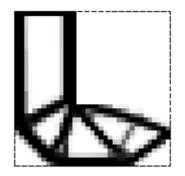
Figure 9. Duysinx and Sigmund (1998) result for a p-mean local stress constraint
