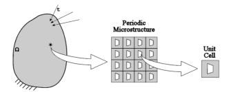
Figure 1. Representation of a composite material made of a periodic microstructure
