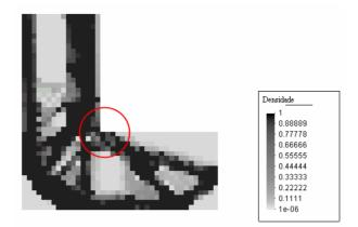
Figure 6. Topology for  $\sigma_1 = 60 \text{ N/m}^2$
