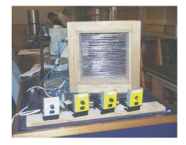
Figure 1. Pictures showing wind tunnel and heating section.
