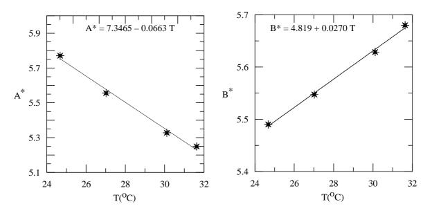
Figure 3. The variation of the calibration parameters  $A^*$  and  $B^*$  with the fluid temperature.
