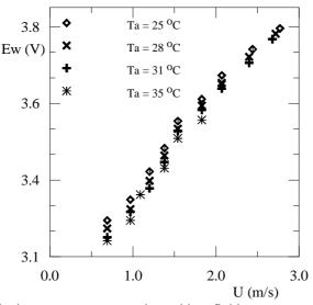
Figure 4. Dependence of velocity measurements on the ambient fluid temperature.
