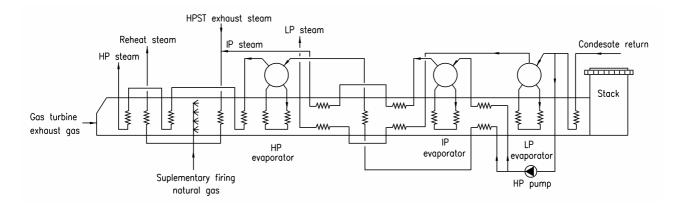
Figure 2. HRSG detailed scheme
