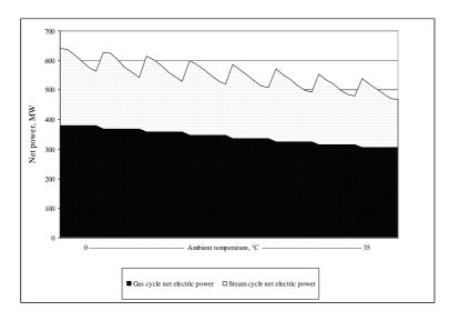
Figure 5. Net electric power generated in the gas and steam cycles
