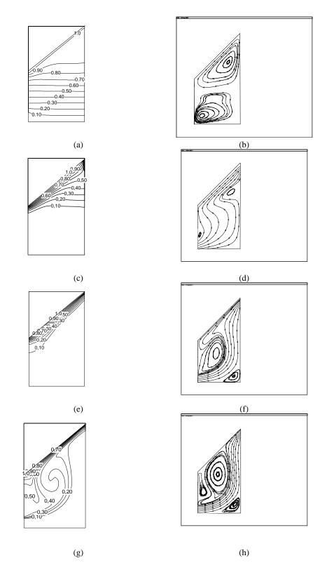
Figure 3 – Isotherms (left) and stream lines (right) for Gr=10<sup>6</sup> and  $\alpha = 45$  for Re=0 (a, b); Re=100 (c,d); Re=500 (e,f); Re=1500 (g,h).
