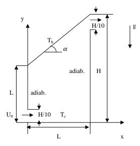
Figure 1. The vented enclosure and the coordinate system
