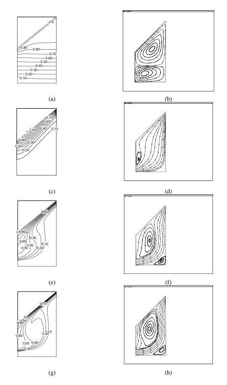
Figure 2 – Isotherms (left) and stream lines (right ) for  $Gr=10^5$  and  $\alpha = 45$  for Re=0 (a, b); Re=100 (c,d); Re=500 (e,f); Re=1500 (g,h).
