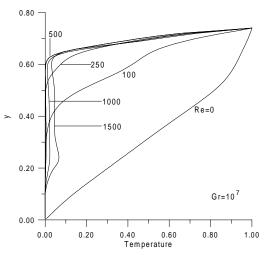
Figure 6. Adimensional temperature along the middle vertical line for some values of the Reynolds number for  $Gr=10^7$ .
