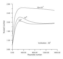
Figure 9. Average normalized Nusselt number in function of Reynolds number for some Gr numbers and  $\alpha = 30^{\circ}$ .
