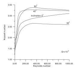
Figure 12. Average normalized Nusselt number in function of Reynolds number for various inclinations, for  $Gr=10^7$ .
