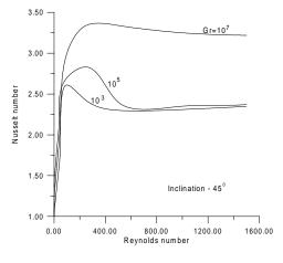
Figure 10. Average normalized Nusselt number in function of Reynolds number for some Gr numbers and  $\alpha = 45^{\circ}$ .
