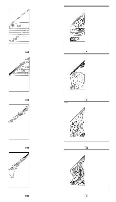
Figure 4 – Isotherms (left) and stream lines (right) for  $Gr=10^7$  and  $\alpha = 45$  for Re=0 (a, b); Re=100 (c,d); Re=500 (e,f); Re=1500 (g,h).
