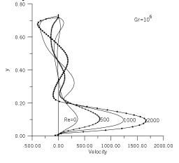
Figure 8. Horizontal components of the velocity along the middle vertical line for values of the Reynolds number.
