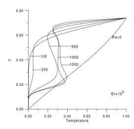
Figure 5. Adimensional temperature along the middle vertical line for some values of the Reynolds number for  $Gr=10^5$ .
