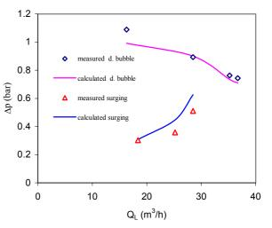
Figure 10. Model Predictions x Experimental Results
