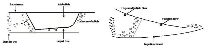
Figure 3. Graphical representation of the observed phenomena - vertical and horizontal cross sections
