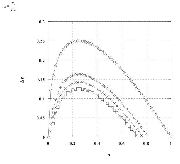
Figure 3. Reduction of the series combined cycle thermal efficiency for the maximization of work output. Symbol O refers to Eq. (14), Other symbols refer to Eq. (30):  $\Box$  is for  $\tau_{int} = 0.6$ ,  $\times$  for  $\tau_{int} = 0.1$  and for  $\tau_{int} = 0.25$ .
