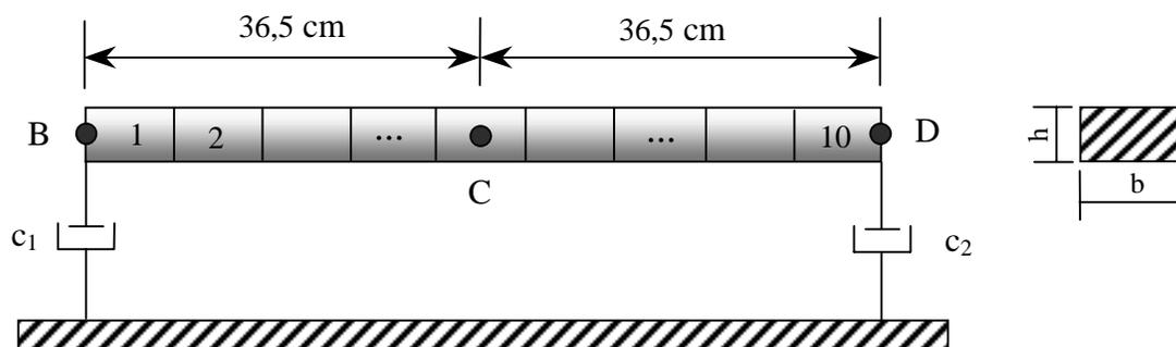
Figure 3 – Characteristics of the FE model of the DVA, divided into 10 macro-elements
