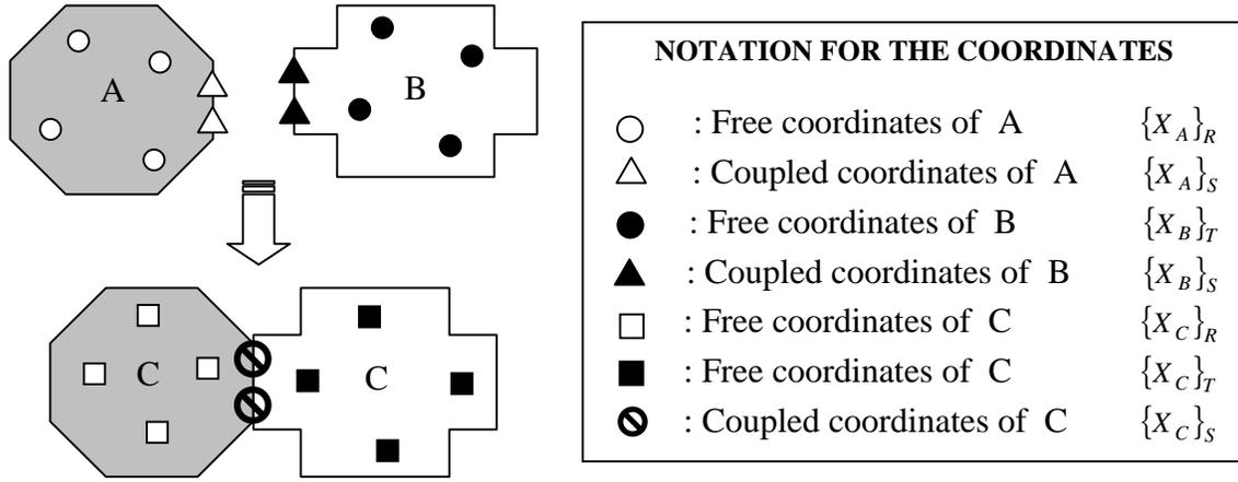
Figure 1 - Coupling of substructures
